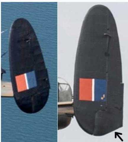
Rudder (right) on the UK's BBMF Lancaster is from a Lincoln. Arrow indicates the shape difference from a Lancaster (on left)
