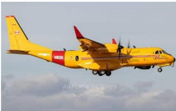
The Kingfisher is powered by two Pratt & Whitney 127G turboprop engines driving six-blade propellers. These engines are in widespread use. They will be much more reliable and will provide the Kingfisher with much greater speed and range than the 50 year old "Buff". The new aircraft will have a highly advanced avionics suite enabling searches to be carried out from higher, safer
